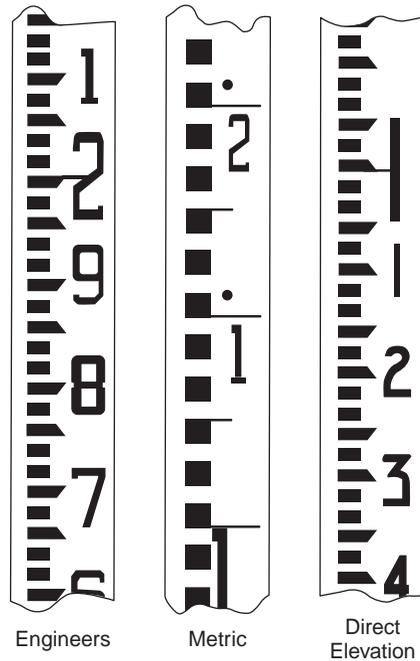
FIGURE 54.8 Typical level rod graduations.
