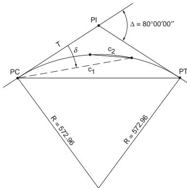
FIGURE 54.29 Horizontal curve layout.
