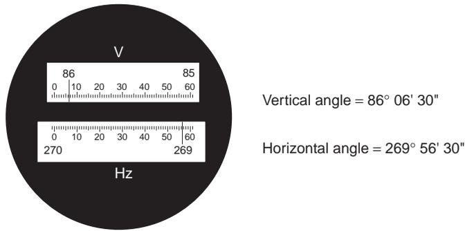
FIGURE 54.17 Scale angle reading display.
