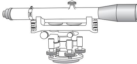
FIGURE 54.5 Engineer's dumpy level.
