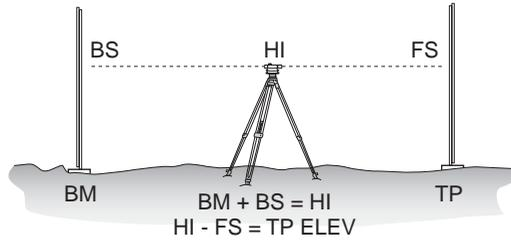
FIGURE 54.9 Differential leveling.
