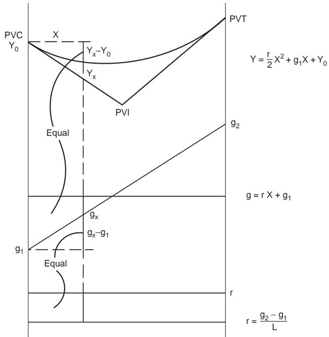
FIGURE 54.30 Sag vertical curve.
