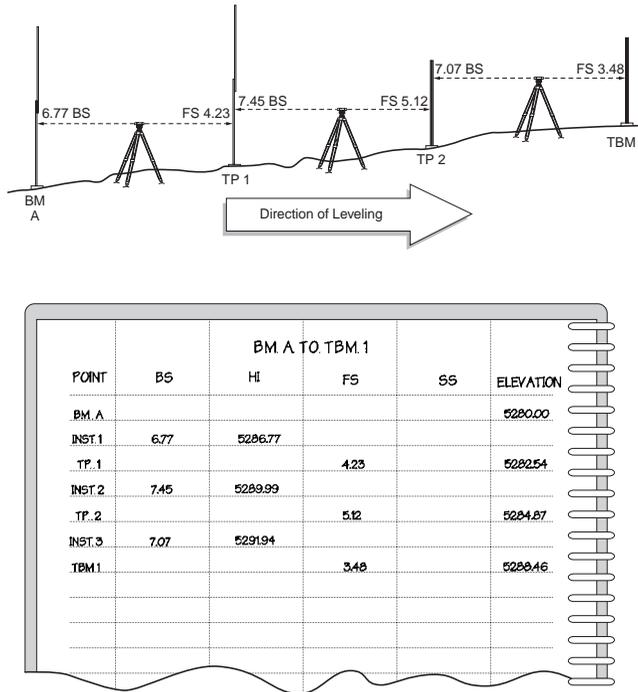
FIGURE 54.10 Level route and field note form.
