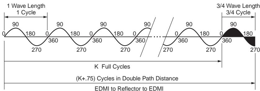
FIGURE 54.2 Phase shift principle of distance measurement.
