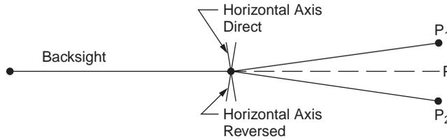
FIGURE 54.21 Double-centering to prolong a straight line.
