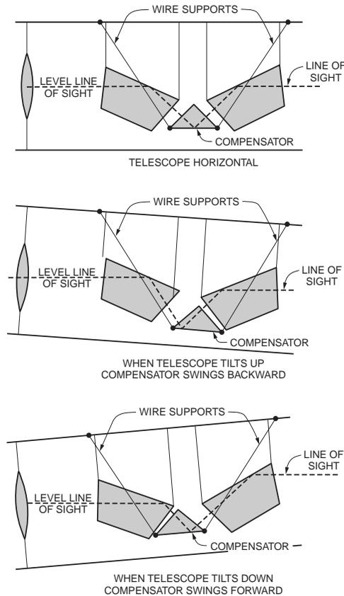
**FIGURE 54.7** Leveling the line of sight by compensator.
