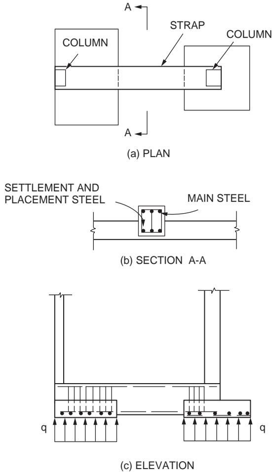
FIGURE 50.27 Strap (cantilever) footing. (Source: Fintel, 1985.)
