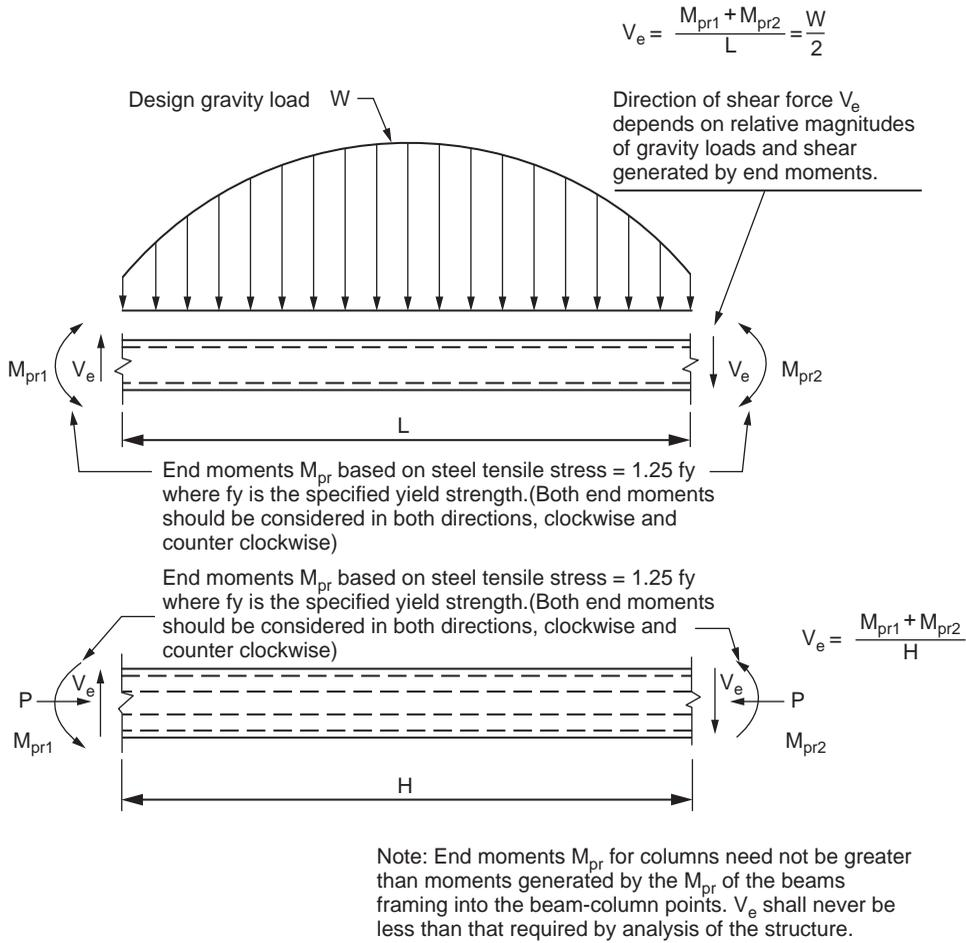
FIGURE 50.12 Design shears for girders and columns. (Source: ACI 318, 1992.)
