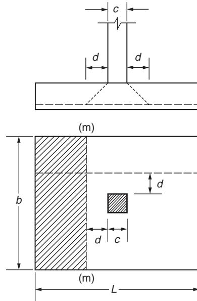
**FIGURE 50.19** One-way shear. (Source: MacGregor, 1992.)
