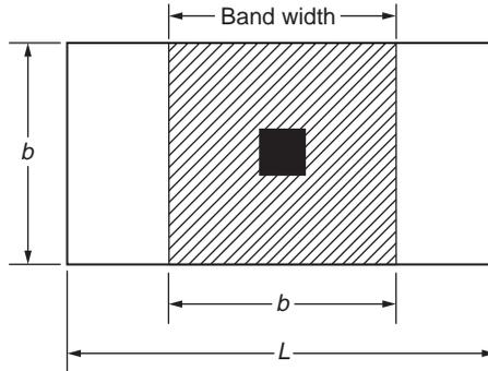
**FIGURE 50.21** Band width for reinforcement distribution. (Source: MacGregor, 1992.)
