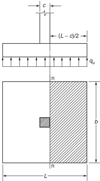
**FIGURE 50.20** Critical section of bending moment. (Source: MacGregor, 1992.)
