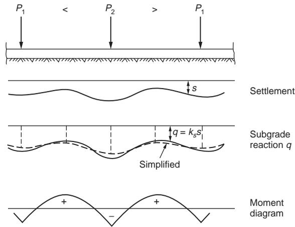
FIGURE 50.28 Strip footing. (Source: Fintel, 1985.)
