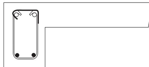
FIGURE 50.4 Stirrup detailing requirements. (Source: Wang and Salmon, 1985.)
