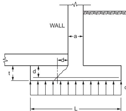
FIGURE 50.23 Reinforced-concrete wall footing. (Source: Wang and Salmon, 1985.)
