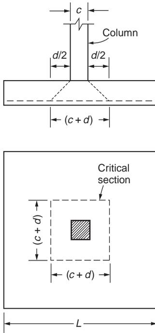
**FIGURE 50.18** Punching shear (two-way). (Source: MacGregor, 1992.)
