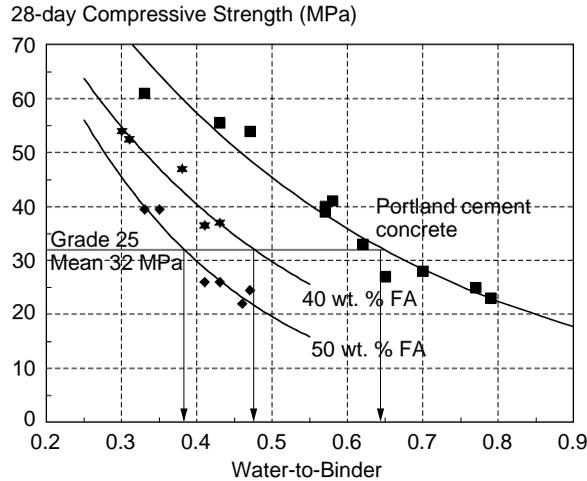
FIGURE 42.8 28-day compressive strength to water-to-binder ratio relationship.
