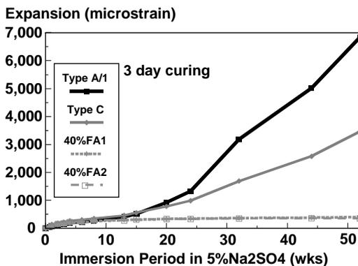
FIGURE 42.19 Expansion of mortar bars in 5% Na<sub>2</sub>SO<sub>4</sub> solution to ASTM C1012 but with 3 days moist curing.
