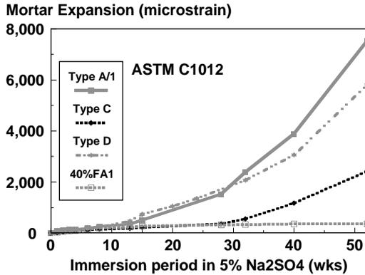
FIGURE 42.18 Expansion of mortar bars in 5% Na<sub>2</sub>SO<sub>4</sub> solution to ASTM C1012.
