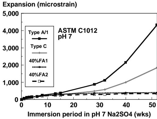
FIGURE 42.20 Expansion of mortar bars in a 5% Na<sub>2</sub>SO<sub>4</sub> solution (low pH 7) to ASTM C1012.
