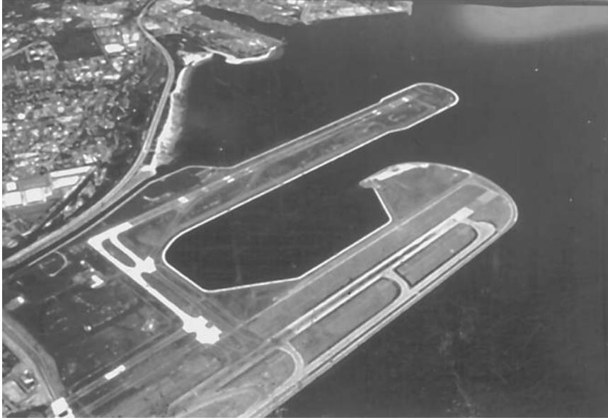
FIGURE 42.7 Aerial picture of seawall around Sydney Parallel Runway, Australia.
