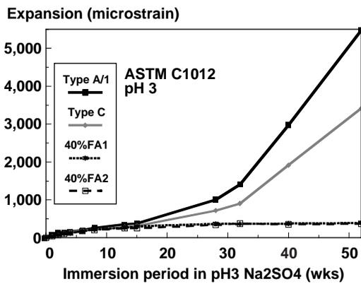
FIGURE 42.21 Expansion of mortar bars in a 5% Na<sub>2</sub>SO<sub>4</sub> solution (low pH 3) to ASTM C1012.
