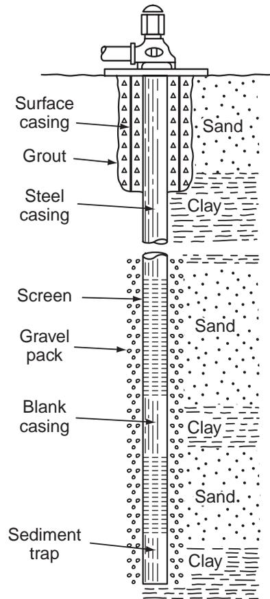
FIGURE 34.6 Supply well with multiple screen and gravel pack. (Source, Heath, R.C., 1998. *Basic Ground-Water Hydrology*. U.S. Geological Survey Water Supply Paper 2220, U.S. Government Printing Office.)
