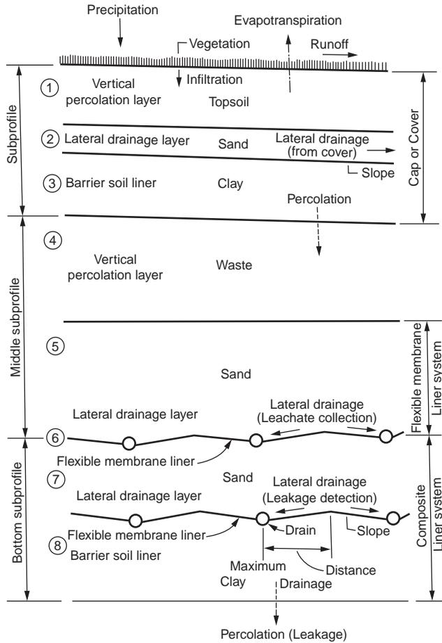
**FIGURE 34.11** Landfill profile. (Source, Schroeder, P.R., Peyton, R.L., McEnroe, B.M., and Sjostro, J.W. 1992a, *Hydrologic Evaluation of Landfill Performance (HELP) Model, vol. III: User's Guide for Version 2*. Department of the Army.)
