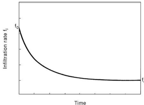
FIGURE 31.6 Infiltration curve.
