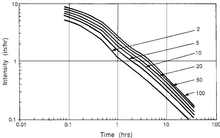
**FIGURE 31.3** Intensity-duration-frequency curves for Indianapolis. (From Purdue, A.M., G.D. Jeong, A.R. Rao [1992] “Statistical Characteristics of Short Time Increment Rainfall,” *Tech. Rept. CE-EHE-92-09*, School of Civil Engineering, Purdue University, W. Lafayette, IN., pp. 64. With permission.)
