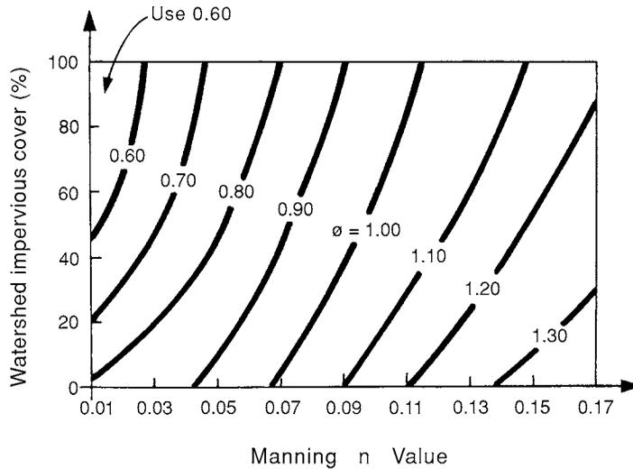
**FIGURE 31.12** Watershed conveyance factor  $\phi$ . (From Espey, W.H., Jr., Altman, D.G. and Graves, C.B., [1977] “Nomographs for Ten-Minute Unit Hydrographs for Small Urban Watersheds,” Tech. Memo 32, *Urban Water Resources*, Res. Prog., ASCE, New York, NY. With permission.)
