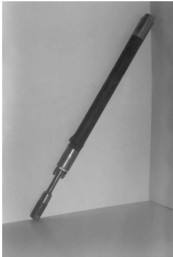
FIGURE 28.2 A pressuremeter. (Picture courtesy of A. Bernal and A. Karim, Bechtel Geotechnical Laboratory, Purdue University.)
