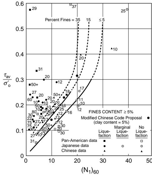
**FIGURE 25.8** Relationship between stress ratios causing liquefaction and  $(N_1)_{60}$ -values for silty sands for  $M_s = 7\frac{1}{2}$  earthquakes (after Seed, H. B., Tokimatsu, K., Harder, L. F., and Chung, R. M. 1985. Influence of SPT Procedures in Soil Liquefaction Resistance Evaluations. *Journal of the Geotechnical Engineering Division*, ASCE. (111) 12:1425–1445).
