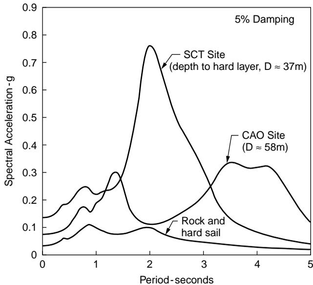
**FIGURE 25.2** Acceleration response spectra for motions recorded in Mexico City during the 1985 Mexico City earthquake (after Seed, H. B., Romo, M. P., Sun, J., Jaime, A., and Lysmer, J. 1987. Relationships between Soil Conditions and Earthquake Ground Motions in Mexico City in the Earthquake of Sept. 19, 1985. Earthquake Engineering Research Center, Report No. UCB/EERC-87/15, University of California, Berkeley).
