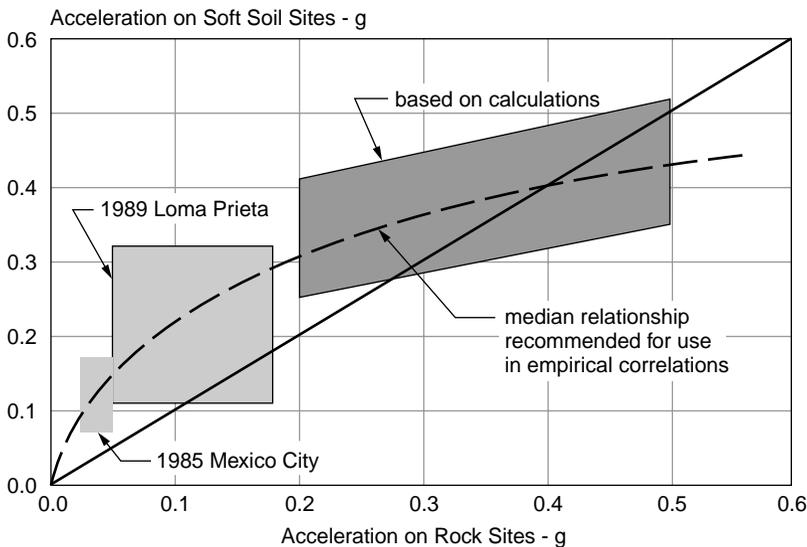
**FIGURE 25.6** Variations of peak horizontal accelerations (MHA) at soft soil sites with accelerations at rock sites (after Idriss, I. M. 1991. Earthquake Ground Motions at Soft Soil Sites. *Proceedings, Second International Conference on Recent Advances in Geotechnical Engineering and Soil Dynamics*, March 11–15, St. Louis, pp. 2265–2272).
