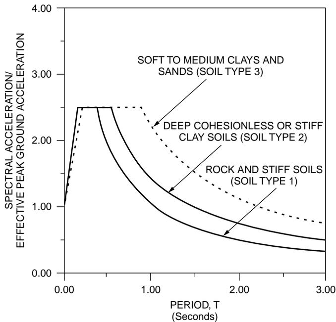
**FIGURE 25.3** 1991 UBC normalized acceleration response spectra.
