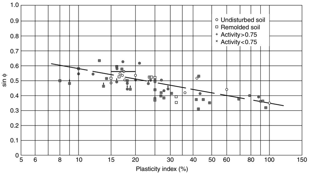
**FIGURE 17.4** Friction angle of fine grained soil based on effective stresses versus plasticity index [Kenney, 1959]. (Source: Lambe, T. C., and Whitman, R. V. 1969. *Soil Mechanics*, p. 307. John Wiley & Sons, Inc. New York. Copyright © 1969.)
