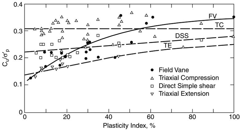
**FIGURE 17.6** Undrained shear strength from  $K_v$  consolidated CU triaxial compression, triaxial extension, and direct simple shear tests as well as field vane tests. (Source: Mesri, G. 1989. A reevaluation of  $s_{u(mob)} = 0.22 \sigma'_p$ . *Canadian Geotechnical J.* 26(1): 163. With permission.)
