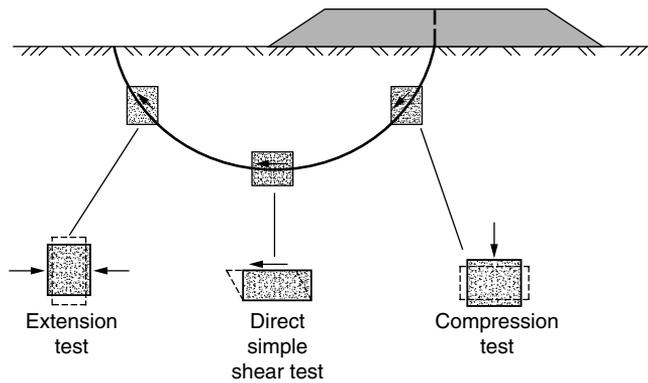
**FIGURE 17.7** Relevance of laboratory shear tests to shear strength in the field. (Source: Bjerrum, L. 1972. Embankments on soft ground. In *Performance of Earth and Earth-Supported Structures*, Vol. II, p. 16. ASCE, New York. With permission of ASCE.)
