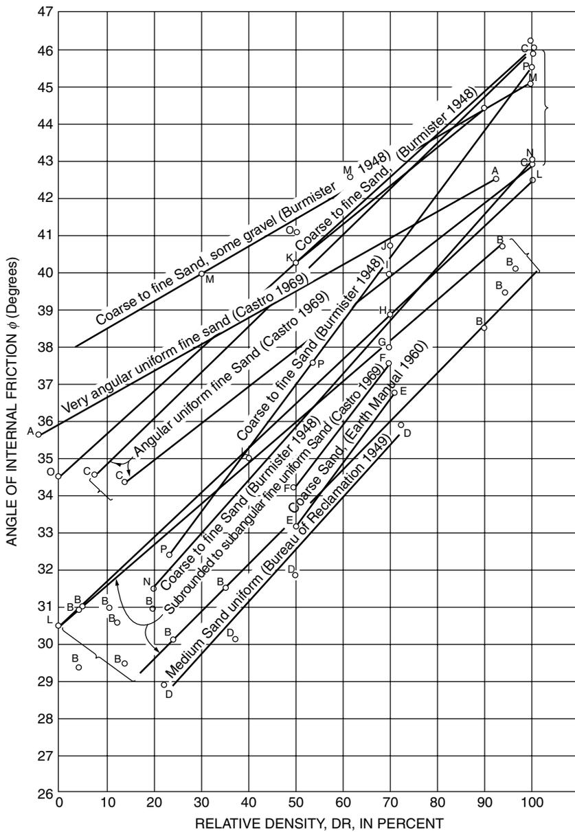
**FIGURE 17.3** Friction angle versus relative density for cohesionless soils. (Source: Hilf, J. W. 1991. Compacted fill. In *Foundation Engineering Handbook*, ed. H. -Y. Fang, p. 268. Van Nostrand Reinhold, New York. With permission.)
