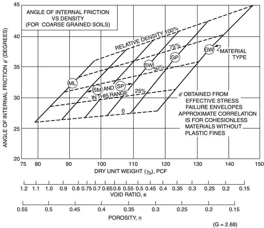
**FIGURE 17.2** Correlation of friction angle of granular soils with soil classification and relative density. (Source: U.S. Navy, 1986. *Soil Mechanics*, Design Manual 7.1, p. 7.1-149. Naval Facilities Engineering Command, Alexandria, VA.)
