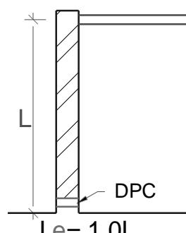
Vertical load resistance of wall or column per unit length:
