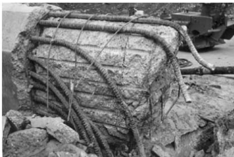
FIGURE 30.36 Failure of connection of column to footing.
