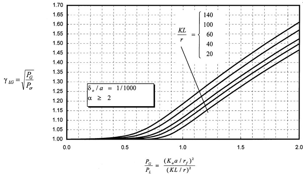
FIGURE 16.23: Buckling mode interaction factor  $\gamma_{LG}$  for  $\delta_0/a = 1/1000$ .
