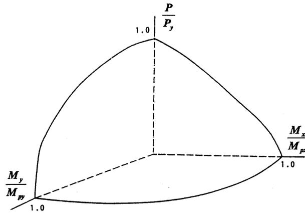
FIGURE 16.30: Typical yield surface for doubly symmetrical sections.
