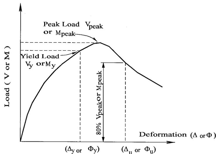
FIGURE 16.26: Load-deformation curves.
