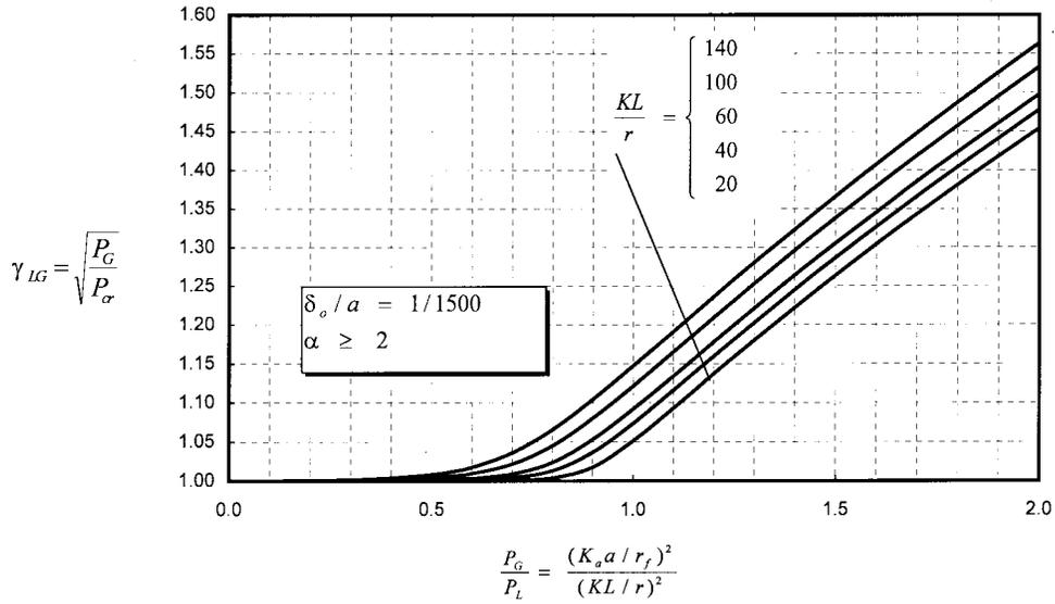
FIGURE 16.24: Buckling mode interaction factor  $\gamma_{LG}$  for  $\delta_0/a = 1/1500$ .
