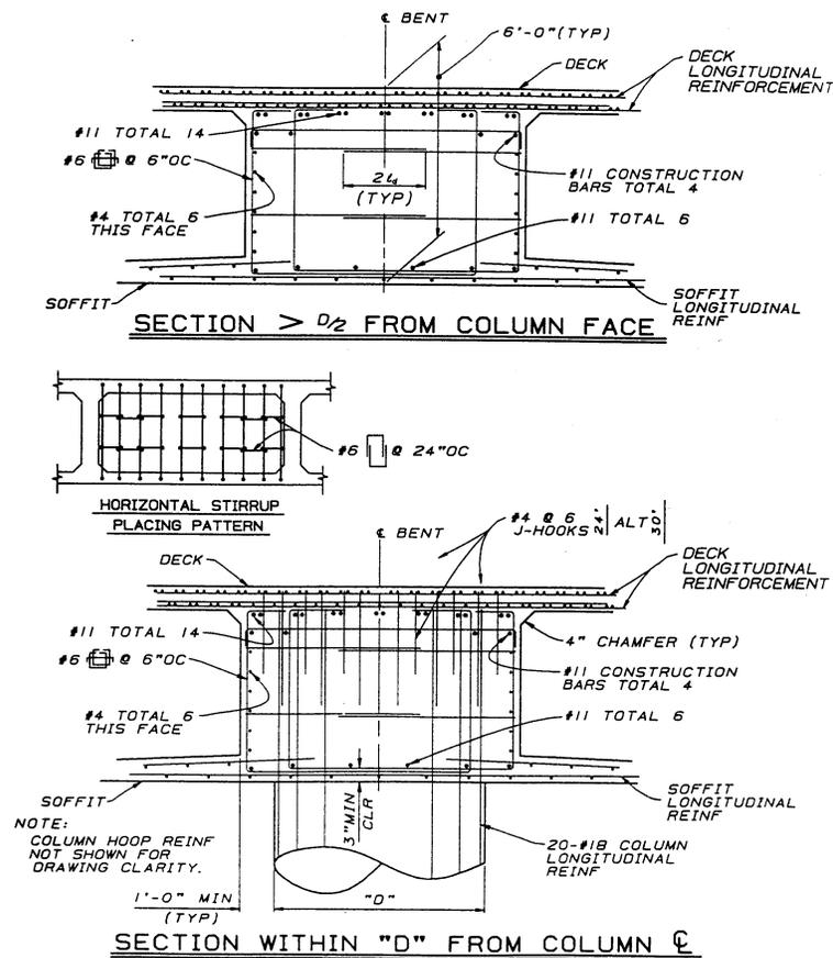
FIGURE 16.18: Example cap joint shear reinforcement — skews > 20°.
