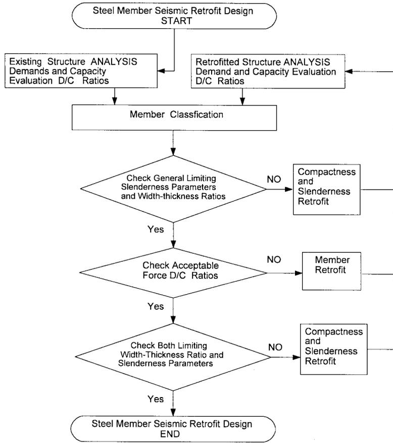
FIGURE 16.15: Steel member seismic retrofit design procedure.
