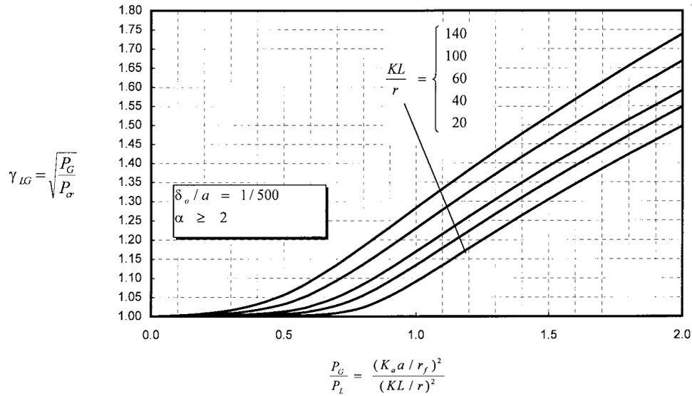
FIGURE 16.22: Buckling mode interaction factor  $\gamma_{LG}$  for  $\delta_0/a = 1/500$ .
