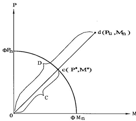
FIGURE 16.25: Definition of force D/C ratios for combined loadings.
