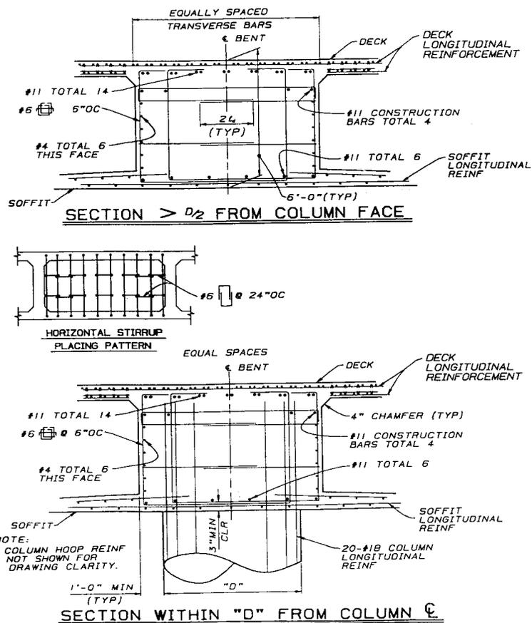
FIGURE 16.17: Example cap joint shear reinforcement — skews 0° to 20°.
