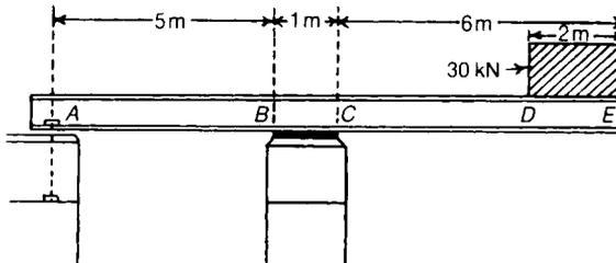
**7.12** Draw the bending moment and shearing force diagrams for the beam shown. The beam is supported horizontally by the strut *DE*, hinged at one end to a wall, and at the other end to the projection *CD* which is firmly fixed at right angles to *AB*. The beam
