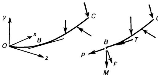
Fig. 7.17 Lateral loading of a curved beam.
