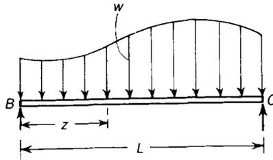
Figure 7.13 Simply-supported beam with lateral load of varying intensity.
