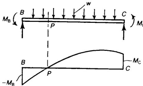
Figure 7.10 Single point of inflection in a beam.
