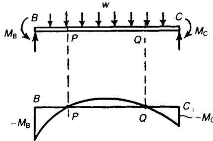
Figure 7.11 Beam with two points of inflection.
