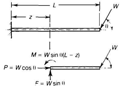
**Figure 7.2** Cantilever with an inclined end load.
