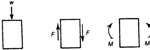
**Figure 7.4** Positive values of  $w$ ,  $F$  and  $M$ , (i) downward vertical loading, (ii) clockwise shearing forces, (iii) sagging bending-moment.
