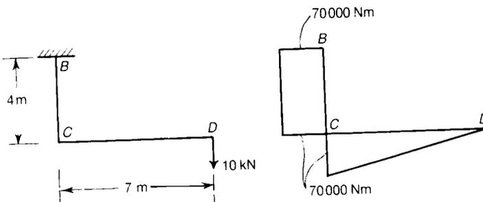
Figure 7.16 Bending moments in a bracket.
