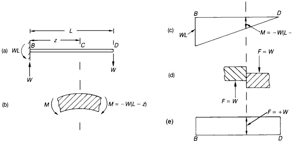
**Figure 7.5** Bending-moment and shearing-force diagrams for a cantilever with a concentrated load at the free end.
