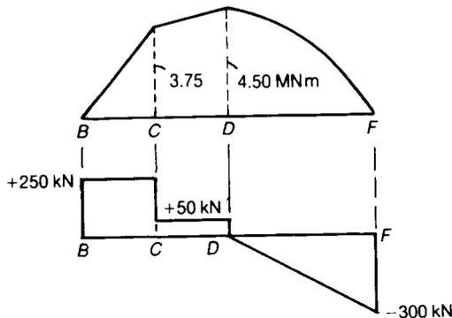
**Problem 7.4** A beam rests on knife-edges at each end, and carries a clockwise moment  $M_B$  at  $B$ , and an anticlockwise moment  $M_C$  at  $C$ . Construct bending moment and shearing force diagrams for the beam.
