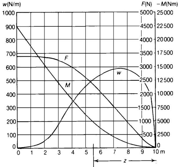
**Problem 7.2** A cantilever of length 10 m, built in at its left end, carries a distributed lateral load of varying intensity  $w$  N per metre length. Construct curves of shearing force and bending moment in the cantilever.
