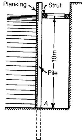
Assuming that the thrust in the strut is two-sevenths the total water pressure resisted by each pile, sketch the form of the bending moment and shearing force diagrams for a pile. Determine the magnitude of the bending moment at  $A$  and the position of the section which is free from bending moment. (Cambridge)
