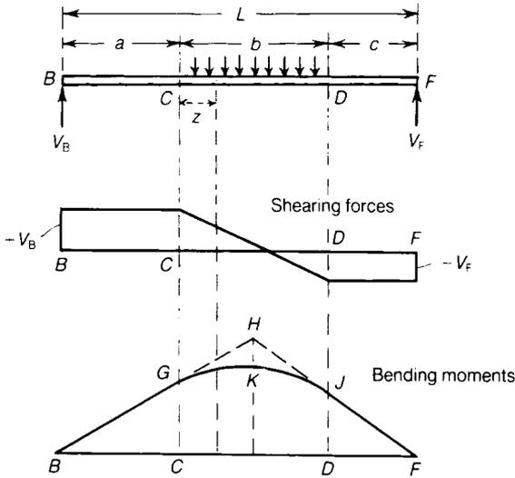
**Figure 7.12** Shearing-force and bending-moment diagrams for simply-supported beam with distributed load over part of the span.
