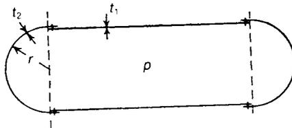
**Figure 6.7** Cylindrical shell with hemispherical ends, so designed as to minimise the effects of bending stresses.
