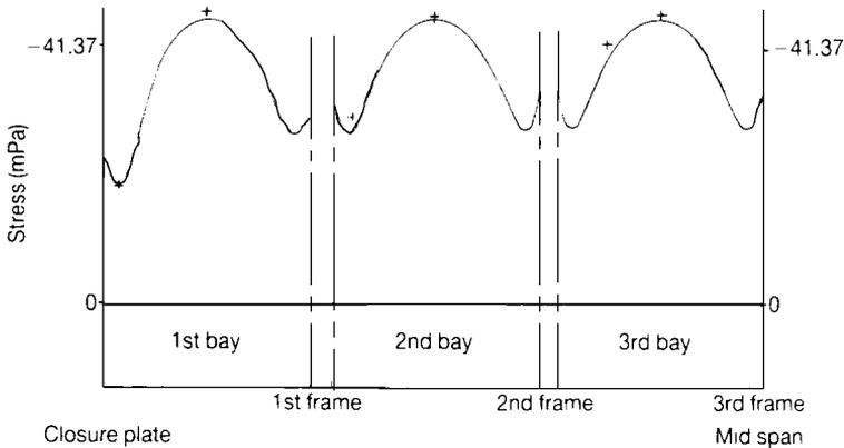
**Figure 6.13** Circumferential stress of the innermost fibre at 0.6895 MPa (100 psi), Model No.2.
