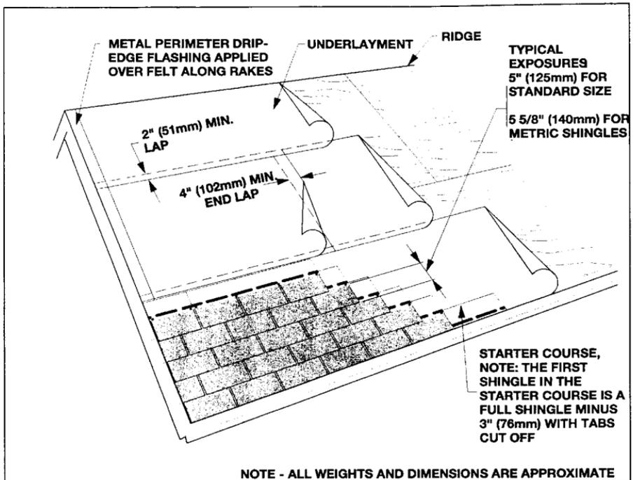
FIGURE 12.7 Three-tab asphalt-shingle roof.
