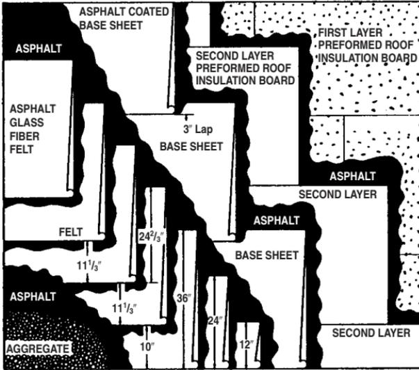
**FIGURE 12.1** Built-up roofing over two layers of preformed insulation board. Three plies of asphalt-impregnated glass-fiber felt, embedded in a continuous application of hot asphalt, overlay a base sheet adhered with asphalt to the insulation. Aggregate surfacing, about  $\frac{3}{8}$  in in diameter, is spread in the top flood coat of asphalt. (NRCA Roofing and Waterproofing Manual.)
